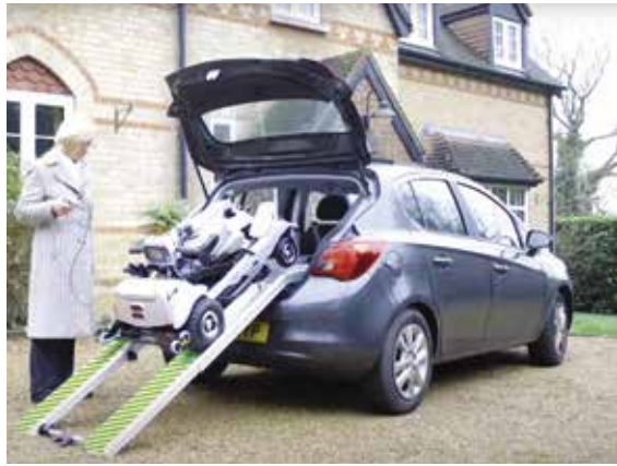
The Quingo Flyte can be loaded and unloaded from a car using a remote control
